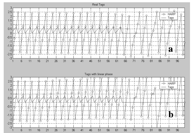
Figure 5. The change in Harmonic Phase signal due to the presence of the linear phase where (a) shows the Harmonic phase signal overlaid on the original real signal while (b) shows the Harmonic phase signal overlaid on the signal suffering inhomogeneity.
