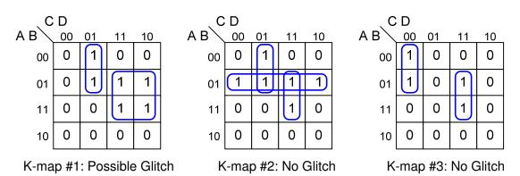
A glitch can be identified in a logic equation if two or more terms include the same logic signal, and the signal is inverted in one term but not in another. For this discussion, each pair of terms that contain a single variable that is inverted in one term but not the other are called "coupled terms", the inverted/non-inverted variable the "coupled variable", and the set of all other variables in both terms the "residue". The examples below illustrate.
