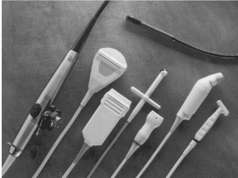
Figure 10.9 Transducer family portrait. From left to right, transesophageal array with positioning assembly, convex (curved) linear array, linear array, stand alone CW Doppler probe, phased array, transthoracic motorized rotatable phased array, and high-frequency intraoperative linear array (courtesy of Philips Medical Systems).
